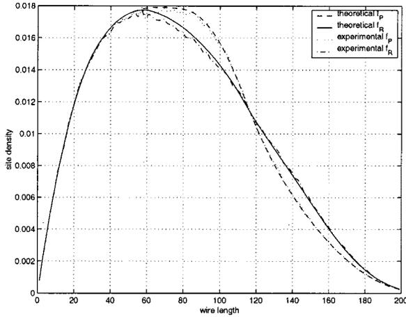
Fig. 9. Experimental verification of the site functions for point redistribution and resultant wires in a C-shaped layout region.
