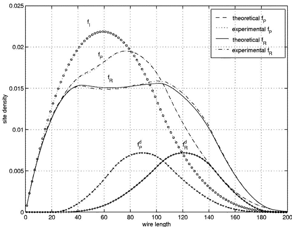
Fig. 3. Site functions with a  $20 \times 80$  obstacle located at the center of the layout region. (a)  $f_I$  for intrinsic wires. (b)  $f_P$  for point redistribution wires. (c)  $f_R$  for resultant wires. (d)  $f_P^d = \sum_{\ell_d} f_P^d(\ell_d)$  for the subset of point redistribution wires that need a detour. (e)  $f_R^d = \sum_{\ell_d} f_P^d(\ell_d)$  with all wirelengths augmented with  $\ell_d$  for the subset of resultant wires with a detour.
