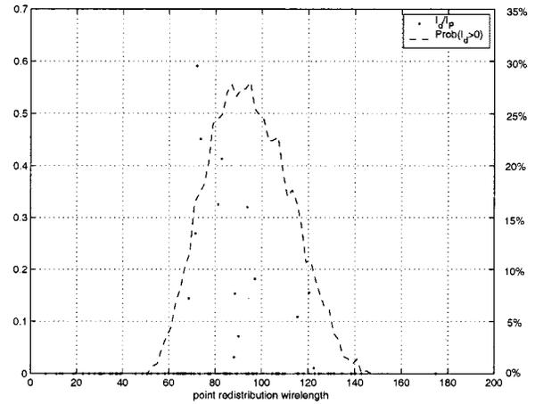
Fig. 10. Detour for different point redistribution wirelengths: each dot is the ratio of detour length  $\ell_d$  over point redistribution wirelength  $\ell_p$  of an individual wire, which values are shown on the left side; the dashed line is percentages of wires that take detour for each point redistribution wirelength, which values are shown on the right side.
